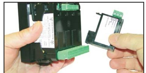
The versatile plug-in units for RS485 (Modbus protocol) and relay option can be purchased with the meter or can be retrofitted at a later time.
