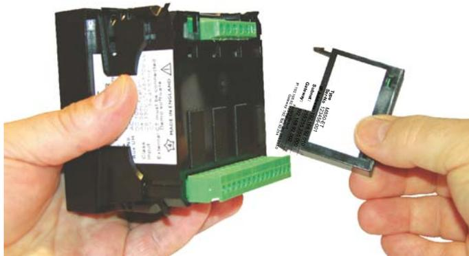
The Ethernet pod (option) can be installed into either position in the back of a M850 power meter. The pod incorporates a 10/100Base-T Ethernet controller.
