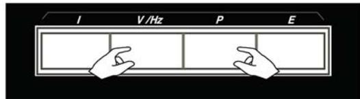
The LED brightness is adjusted by holding down the two center buttons.
